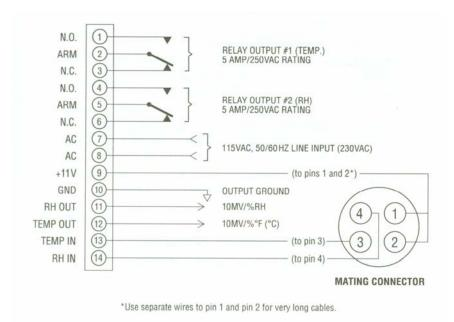
**NOTE:** Recorder output devices should share the same ground as Terminal No. 10.
